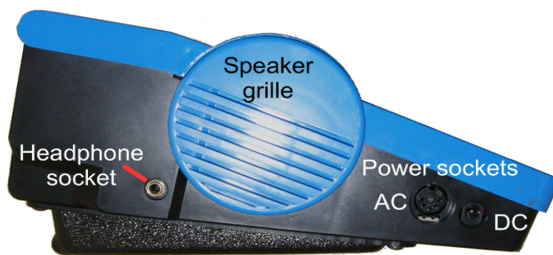
Illustration 6: The left side of the MB W+, showing the sockets and speaker grille
