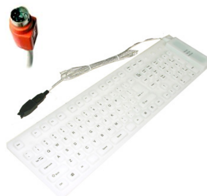
Illustration 15: PC keyboard showing the PS/2 connector
