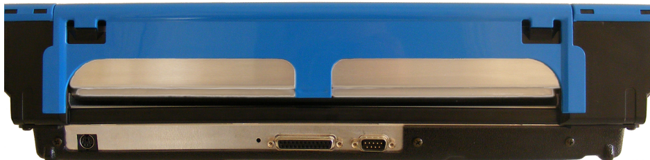
Illustration 8: The rear of the MB W+, showing the ports
