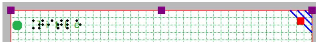
Figure 1. The top of the design shows the title text label, right-up marker and red border for paper size and orientation.
